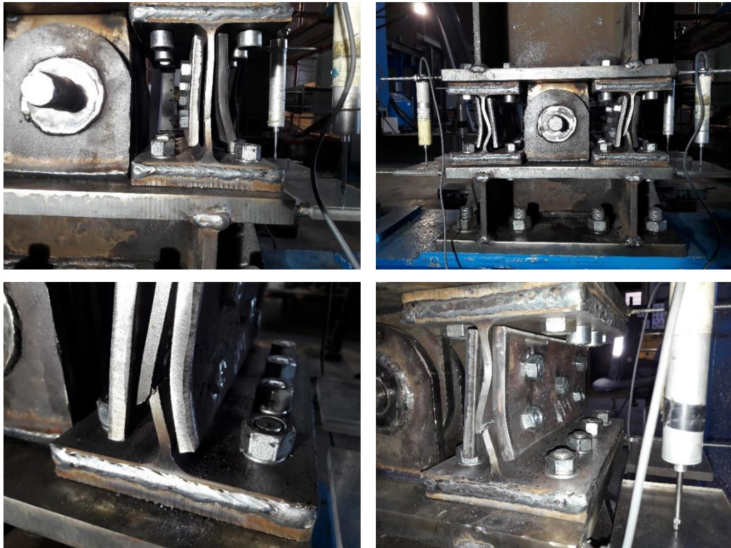
Figure 3.37: Permanent deformations and damages after PT4 Test
