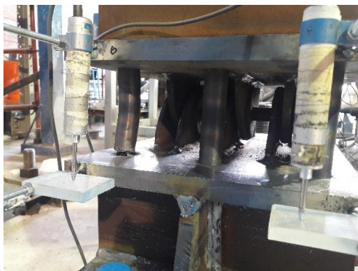
Figure 3.10: Permanent deformations and rupture of T/C bars after Test #1
