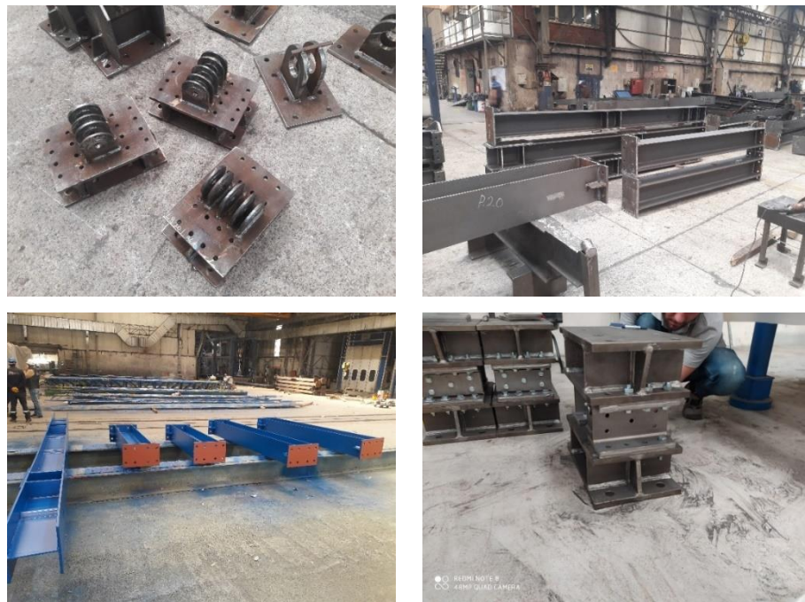
Figure 4.3: Production of P-Cells and frame members
