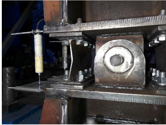
Figure 3.30: Permanent deformations and damages after PT3 Test
