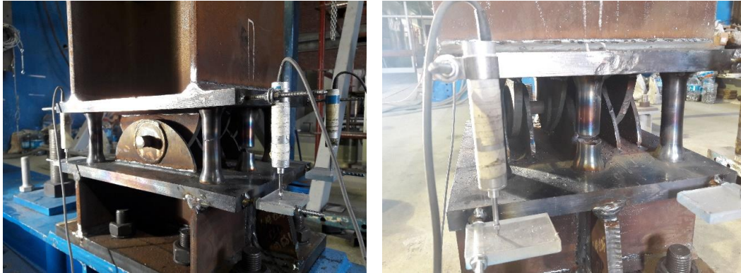
Figure 3.16: Permanent deformations and damages after PT2A Test
