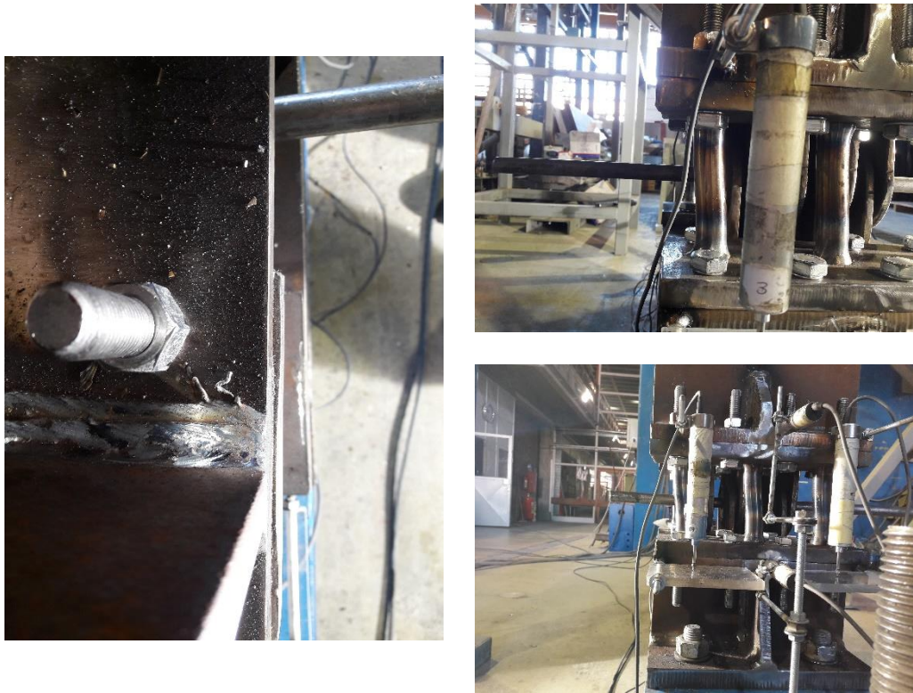
Figure 3.23: Observed torsional behavior on PT2B
