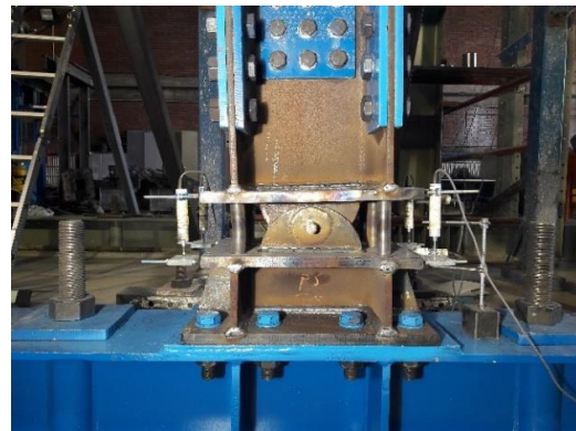
Figure 3.9: Observed deformations on PT1 during Test #1 at different top displacement levels
